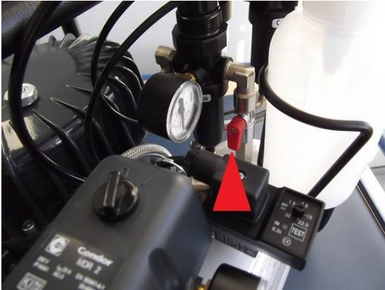
Fig. 4 Turn the tap in the open position (in line with the air flow).
