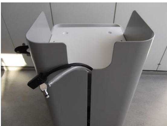
Fig. 9 Place the air hose and power cord on top of the trolley, as in the picture, and insert the cable into the clamp. Close the front door of the trolley.
