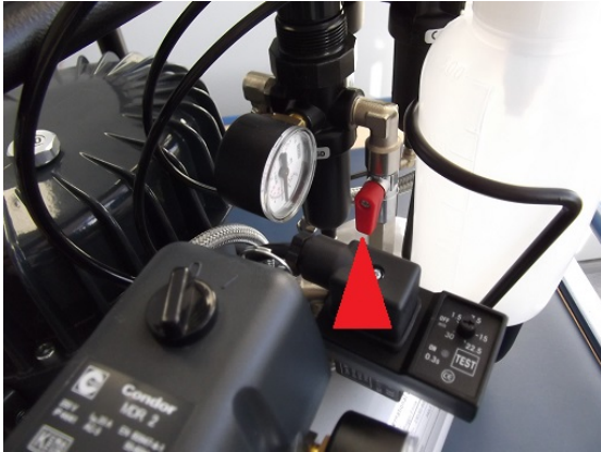
Fig. 4 Open the cut off cock ( the red hand gear is perpendicular)
