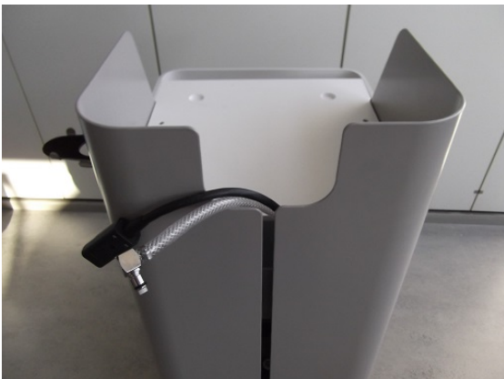
Fig. 9 Lay the air hose and the power cord of the compressor upward. Close the front door of the „Trolley“
